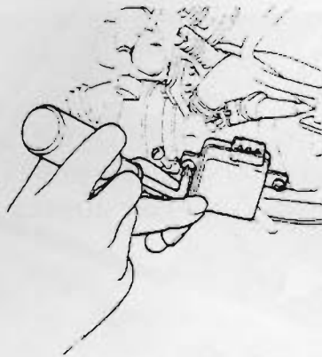
Fig. 5 Loosening the throttle switch screws
