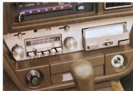
Unusual stereo design means aftermarket DIN units don't fit; originals can be repaired.
