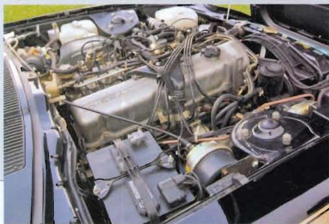
Fuel injected 2.8-liter six carried over from 280Z, and its durability was proven; most engine parts are readily available today.
