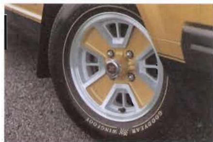
Color-coded alloys exclusive to 10th Anniversary cars; Wingfoot tires no longer available.
